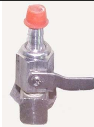
Fuel circuit valve Closed
