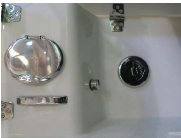
Water tank filler
