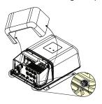
**NOTE**: Use a Philips #2 screwdriver to loosen the captive nut panel screw(s).
