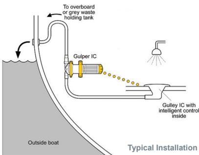
Compact Gulley design senses waste level and controls pump
