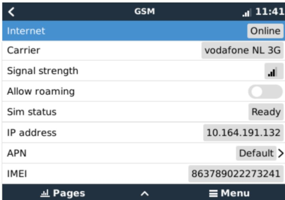
When using a SIM card with its SIM-pin security disabled, the system will work without further configuration.
