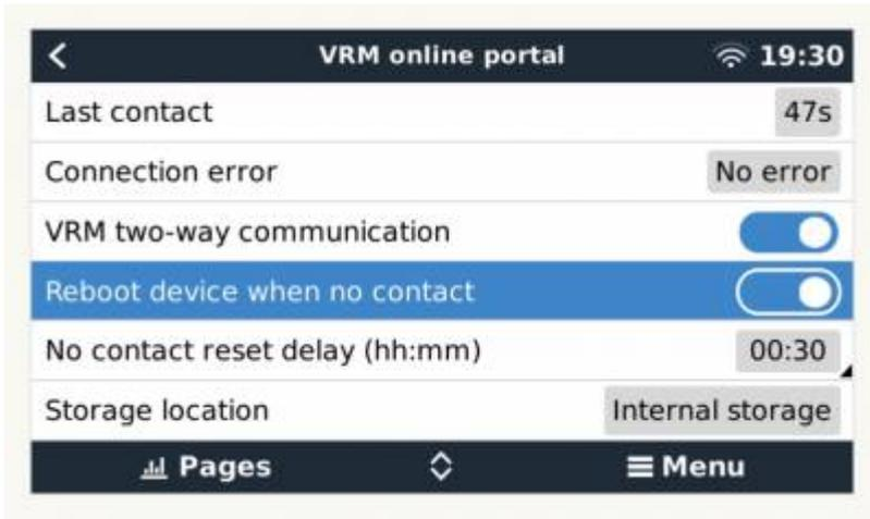
Note that if you are leaving internet service coverage areas (such as an RV on the move, or a boat leaving dock to go to sea) then it is recommend to disable this setting, so that your GX is not rebooting itself for no reason. Or set it, for example, to a two hour time-out. And accept a reboot every two hours when underway.
