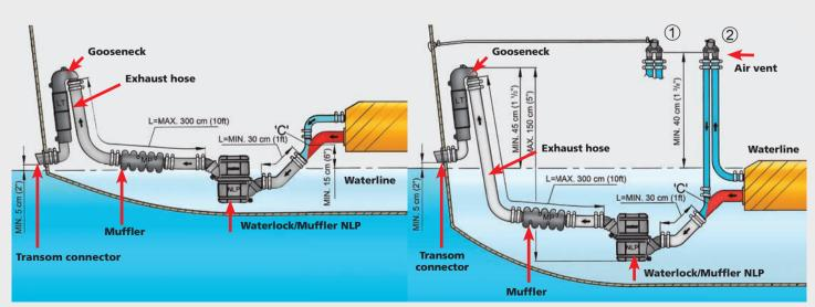
Exhaust system with the water injection point "C" 15 cm (6") or more above the waterline.
