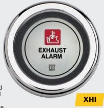
The temperature sensors, to be fitted into the exhaust hose or the waterlock/muffler, and the alarm unit must be ordered separately. In the case of a twin engine installation 2 sensors may be connected to 1 alarm unit, if so required. One sensor may also serve two alarm units, e.g. in the case of a second steering position. Cut-out dimensions: Ø 52 mm (21/16"). Outside dimensions: Ø 62 mm ( $2^{7}/_{16}$ "). Available for 12 and 24 Volt D.C.
