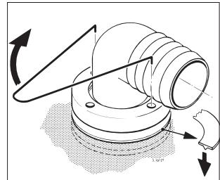
Check after 2 days if the nuts are still properly secured; tighten the nuts if required.
