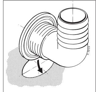
Fit the ring and nut. Tighten the nut with the wrench, never use water pump pliers. Do not tighten too hard.
