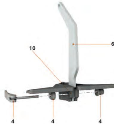
Fig. 57: Control triangle and swing arm
