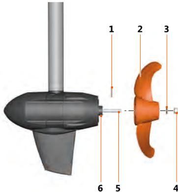
Fig. 85: Propeller attachment for Ultralight 403 A/AC
