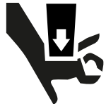
Caution: risk of crushing
