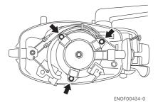
Insert the knotted end of the starter rope into the notch in the flywheel and wind the rope around the flywheel several turns clockwise.
