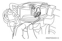
3. Remove the bolts (3 pcs) and remove the recoil starter.
