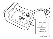
After filling the tank, close the fuel tank cap until two clicks sound is heard. ENOM00037-C
