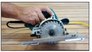
4. Note: Saw safety cap should be put back on before using. Cap was removed only to show blade. A seam saw can be used especially when seam must be deepened to a minimum
