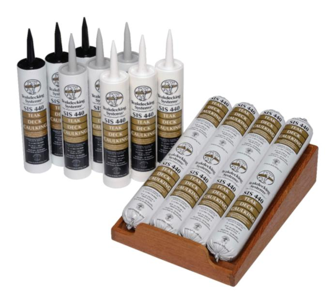
SIS440 Caulk is the proven leader in the marine industry and was developed mainly for teak deck seams. It is a one-part, paste-like neutral cure formulation and when exposed to moisture in the air, it reacts to form a tough, flexible solid rubber compound. The sealant does not sag during cure, and has excellent temperature stability and chemical resistance once cured. Because the sealant is neutral cure, it is non-corrosive to all substrates.
