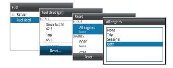
→ *Note:* You can reset the total for one engine or all engines.
