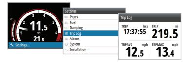
→ *Note:* Trip information is calculated using GPS or the paddlewheel if GPS is not present. No Trip Log information is recorded while the Trip Log is stopped.
