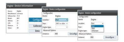
→ Note: Configuring the engine location correctly is important when more than one engine is on the network.
