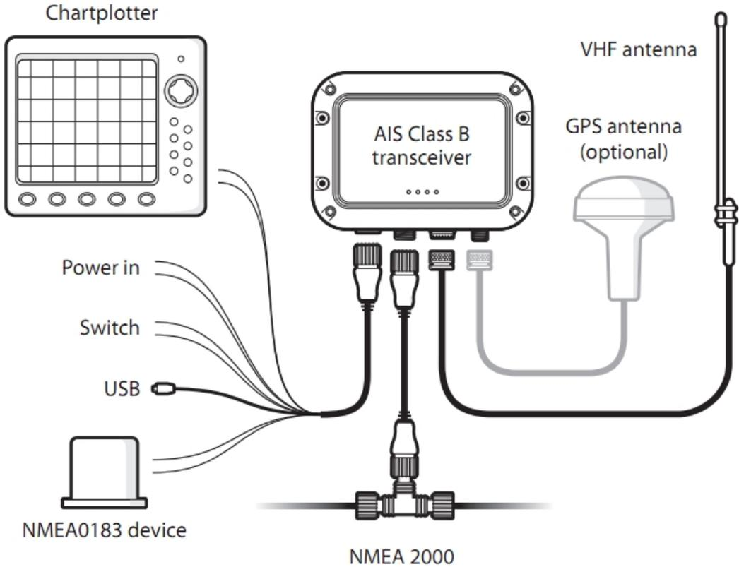
Figure 4 Typical installation configuration
