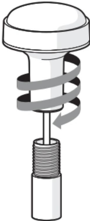
*Figure 7 GPS antenna mounting*
