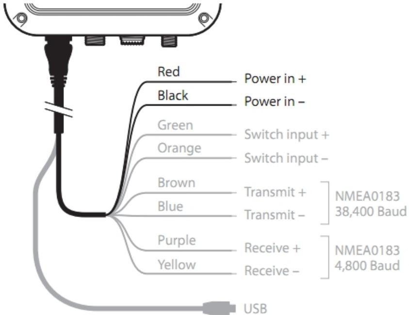
Figure 12 Connecting the power supply
