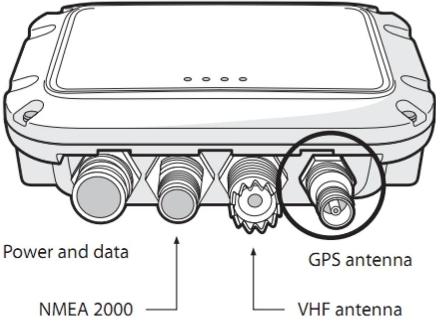
Figure 8 Position of the GPS antenna connector
