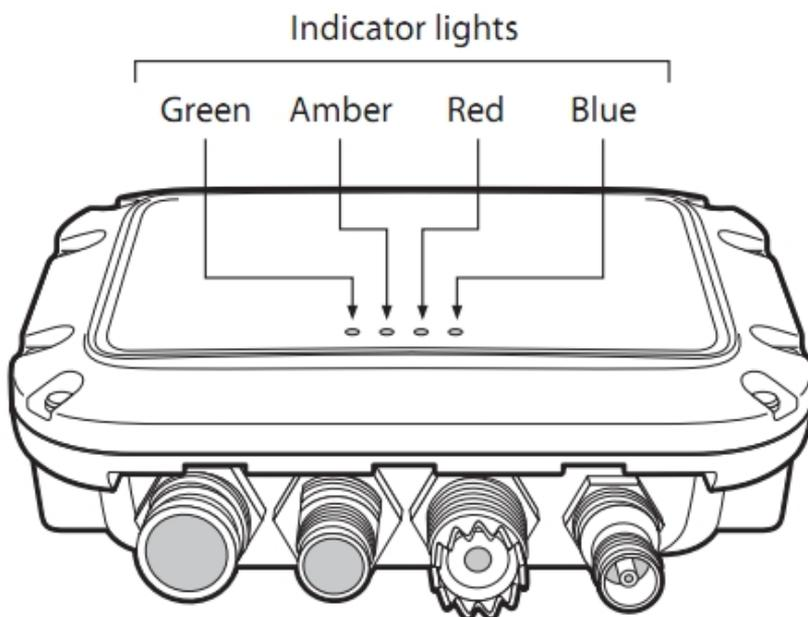
*Figure 14 Indicator location on the AIS transceiver unit*
