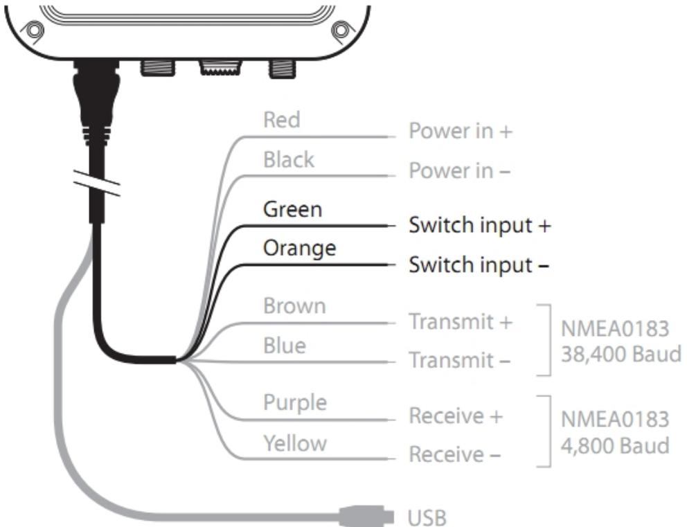
Figure 10 Connecting an external switch
