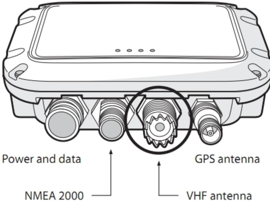
*Figure 9 Position of the VHF antenna connector*
