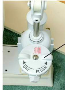
Position for discharge of bowl contents only (no water coming in)
