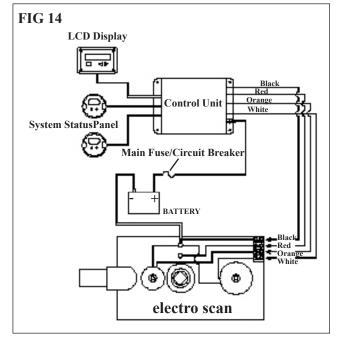
**Note:** Normal installations have one System Status Panel. This diagram depicts a dual system installation
