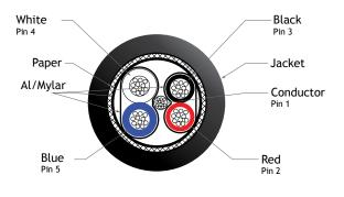
The light pair used for the network power shall be No. 22AWG (0.38 sq. mm) or heavier. The light pair for signals shall have the following electrical characteristics.
