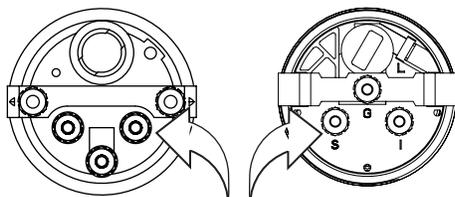
Electrical connections tighten 0.70 Nm max. (100 in. oz.)
