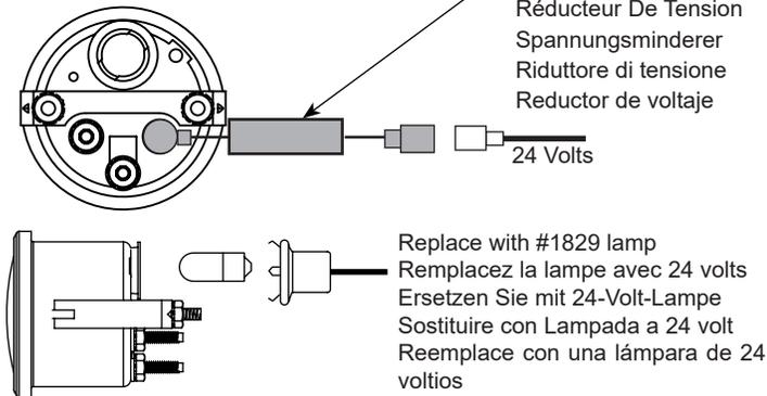
Remove lamp & replace with # 40102E007 and #6283274 socket.
