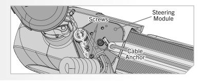
Using a #3 Phillips screwdriver, tighten the Cable Tension Screw located at the base of the Toe End of the Foot Pedal to 10 - 12 in-lbs until the Steering Cables are under tension or re-tighten the same number of turns as was used in step 4f.
