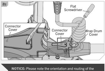
plug and wires for re-installation.
