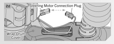
e. Remove the two screws that hold the Wrap Drum Cover in place with a #2 Phillips Screwdriver. Once removed, lift the Wrap Drum Cover away from the Steering Module.
