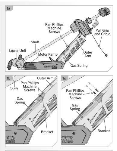
**NOTICE:** Use a #3 Philips Screwdriver to remove the screws. They have a pre-applied thread locker. Failure to use the recommended tool can cause damage and prevent the screws from being removed.
