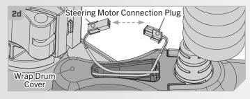
e. Remove the two screws that hold the Wrap Drum Cover in place with a #2 Phillips Screwdriver. Once removed, lift the Wrap Drum Cover away from the Steering Module.
