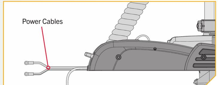
**NOTICE:** The Riptide PowerDrive has no power switch. When the Power Cables are connected to a battery, the Riptide PowerDrive is "on". When the Power Cables are disconnected from the battery, the Riptide PowerDrive is "off". If the Power Cables are connected to a breaker, the Riptide PowerDrive is "on" when the breaker is "on" and "off" when the breaker is "off".
