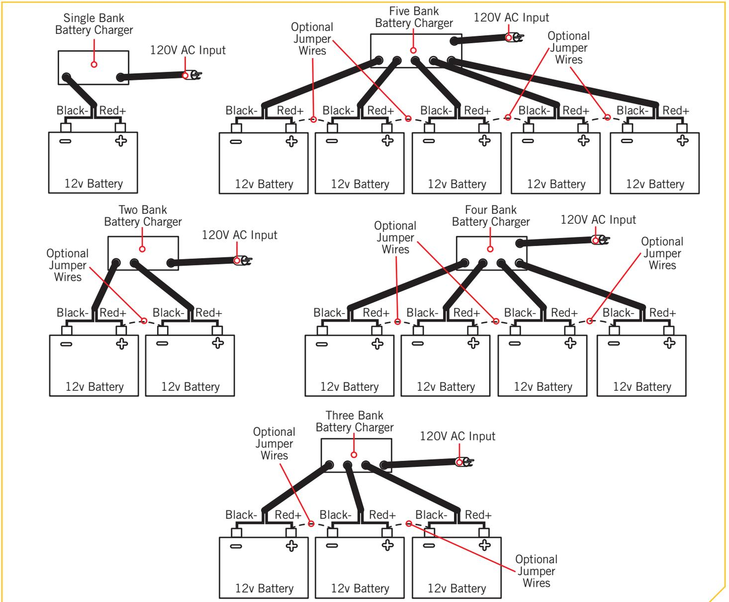
**NOTICE:** If batteries are connected in a series with Jumper Wires, those wires can be left in place during charging.
