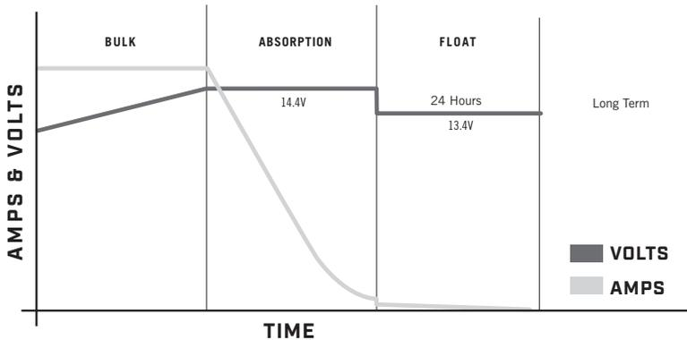
**NOTICE:** In long term storage, the charger will automatically resume the charging process beginning with Bulk Mode when the battery voltage drops below 12.6V.
