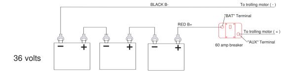
**NOTE:** The 24 / 36 volt diagrams shown here show a series link being made at the batteries. Some installations will have the series link made at the trolling motor plug or plug receptacle.
