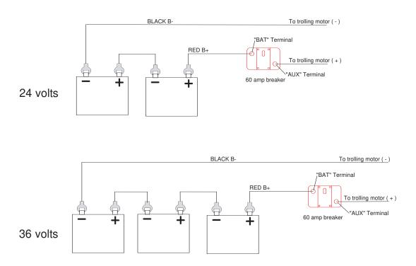
**NOTE:** The 24 / 36 volt diagrams shown here show a series link being made at the batteries. Some installations will have the series link made at the trolling motor plug or plug receptacle.
