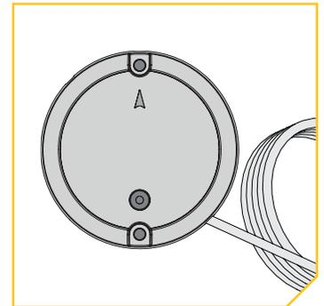
**NOTICE:** If replacement screws must be used, ensure that they are high grade non-magnetic stainless steel.
