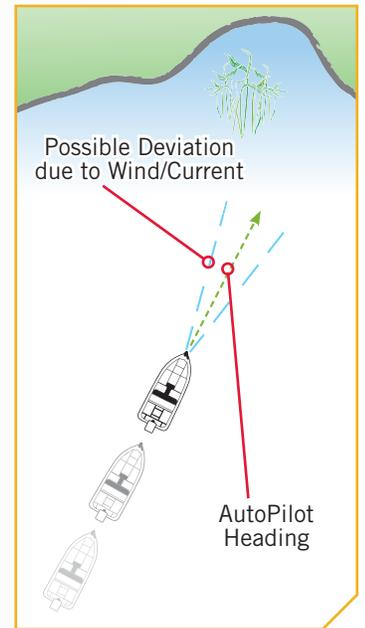
**NOTICE:** After steering to a new direction, there is a short delay before the direction is locked in to allow the compass to stabilize. When broad speed changes are made, the AutoPilot heading may change slightly. This is normal.
