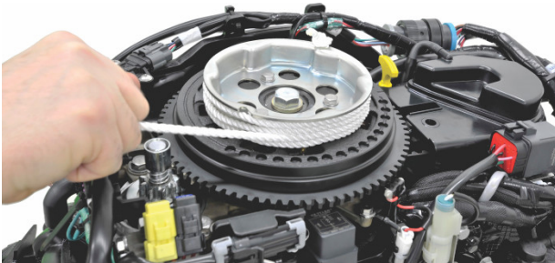
Emergency starter rope on flywheel cup (typical)
