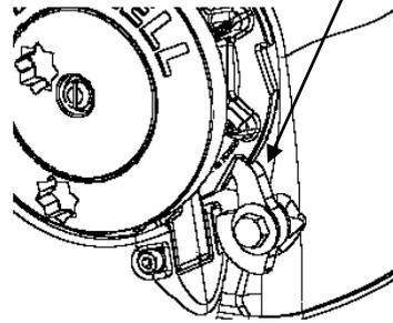
Insert the clutch handle into the clutch nut and turn anticlockwise to loosen the clutch. Note the chain wheel may pay out the anchor until the pawl locks into the chainwheel.
