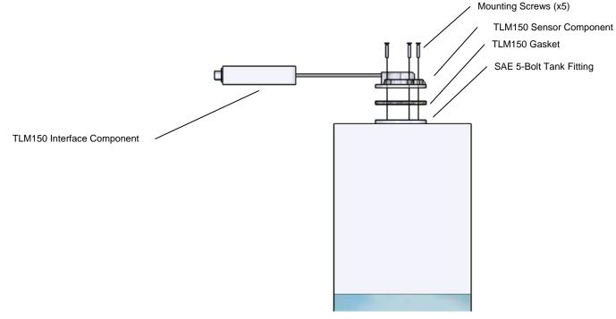
Figure 2 – TLM150 Mounting – SAE 5-Hole Bolt Pattern
