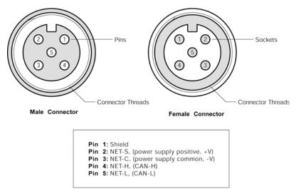
Figure 7 – NMEA 2000<sup>®</sup> Connector Face Views
