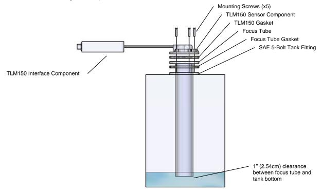
Figure 3 – Mounting TLM150 to SAE 5-Hole Tank with Focus Tube
