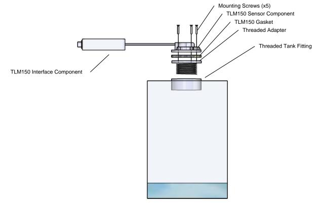
Figure 4 – TLM150 Mounting With Threaded Adapter
