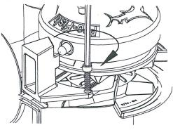
9. Fix Stripper & Cam into place using two new longer screws supplied. Use Loctite (not supplied) on the threads of the screws prior to fitting them. Allow at least <u>15mins</u> for Loctite to cure before use.
