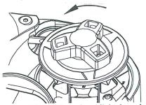
2. Undo the Clutch Nut using 1/2 inch ratchet and or the Pro-Series winch handle & unscrew by hand.
