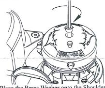
6. Place the Brass Washer onto the Shoulder Screw. Put Loctite (not supplied) onto thread of bolt and fit into the end of the Main Shaft. Tighten up using allen key provided (15Nm, 11lbf/ft). Allow at least 15mins for Loctite to cure before use.
