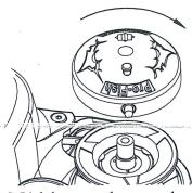
5. Lightly grease the exposed end of the Main Shaft & gypsy / cone interface, making sure you do not get grease in the threaded hole in the end of the shaft. Place Pro-fish Cap assembly onto the Shaft and screw down by hand.
