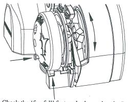
10. Check the 'freefall' feature by loosening the Profish Cap & spinning the Gypsy with your hands. The Gypsy should be able to spin freely.
