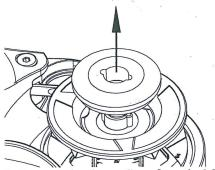
3. Remove the Gypsy Cone from the Main Shaft.
