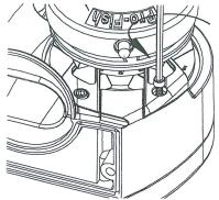
7. Undo & remove Stripper Screws using allen key provided.
