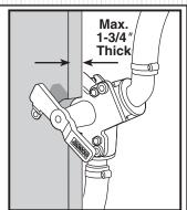
Mounted through bulkhead with optional handle extension.
