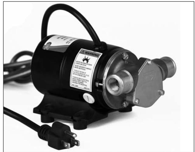
1. **INSTALLATION** – Pump may be mounted at any angle without loss of efficiency. Suggested mounting is horizontal or with pump head down. The inlet port is the right hand port when looking at the end cover.
