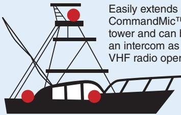
Easily extends up to two CommandMic™ on a tower and can be used as an intercom as well as for VHF radio operation.
