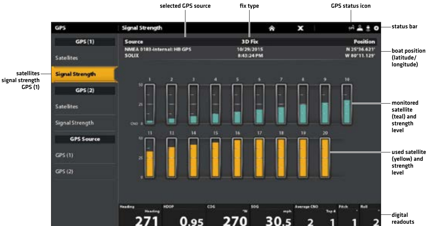
Signal Strength (GPS 1/GPS 2): displays vertical bar graphs indicating the satellite signal strengths with the respecting CNO (Carrier-to-Noise) value (0 to 60).
