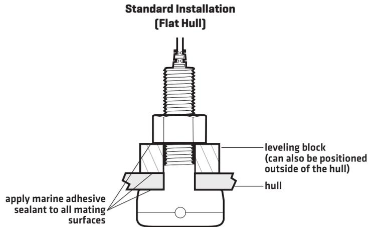
1. From the outside of the hull, drill a small pilot hole [smaller than the centering bit of your drill bit or hole saw], at the mounting location you selected in section 2. **Drill the hole perpendicular to the hull.**
