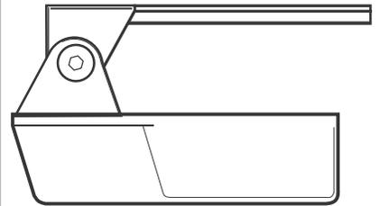
Mounting bracket should be parallel to the transducer.
