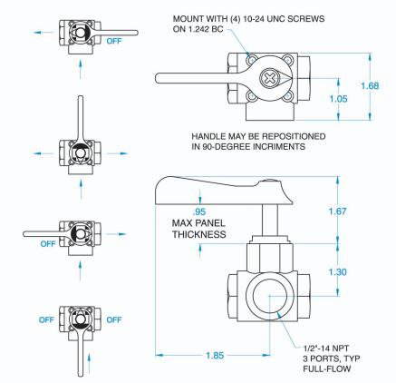
TS-350-T Tank Selector Kit utilizes FV-350-T full flow valve (see above for details) mounted on an attractive stainless steel mount bracket and plumbed with (2) ½" hose barbs and (1) 7/16" hose barb.
