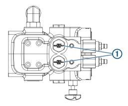
Depending on the model of pump, the check valves are located on either the side or top of the manifold.
