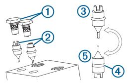
The pump is configured from the factory with the pistons in the balanced configuration ③, where the tip of the piston is pointing into the pump manifold.
