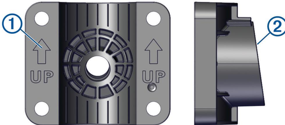
**NOTE:** The trolling motor shaft bracket has an 8-degree angle to reduce the effects of the trolling motor barrel interference with the transducer beam.
