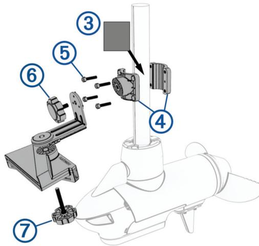
**NOTE:** The rubber liner is not needed when installing the transducer on a trolling motor with a shaft diameter larger than 25 mm (1 in.).
