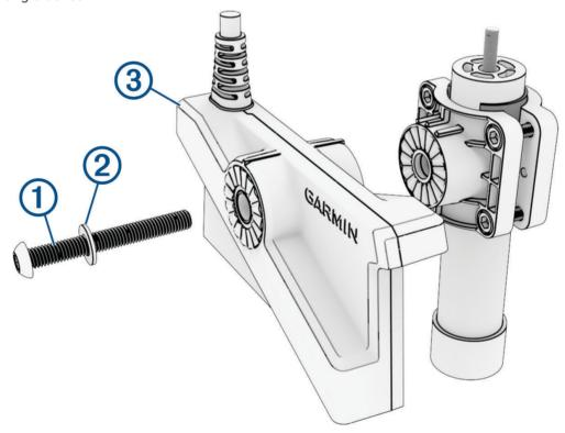
3 Adjust the view of the transducer and tighten the low-profile screw using the included hex wrench.
