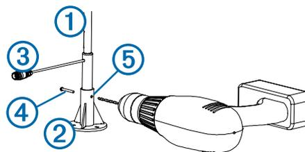
**NOTE:** If you do not mount the device with the cable facing the front of the boat, exactly parallel to the center line, or if you mount the device with the cable facing the back of the boat, you must configure the orientation to receive accurate wind-angle data ([Adjusting the Orientation, page 3](#)).
