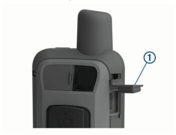
2 Insert the memory card with the gold contacts facing the device screen.
