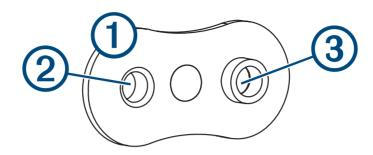
The other hole ③ on the nut plate should line up with the inner 4 mm ( $\frac{5}{32}$  in.) hole on the template.
