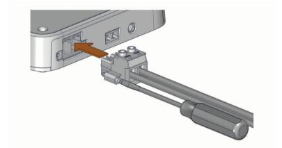
6 Using a 5.5 mm ( $^{7}/_{32}$  in.) flat (slotted) screwdriver, secure the power terminal block to the amplifier.
