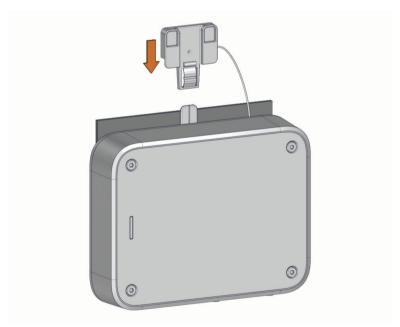
4 Install the included screw covers in the four holes on the top of the amplifier (optional).
