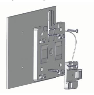
**NOTE:** You must install the bracket with the release tab pointing up to properly secure the amplifier in the bracket.
