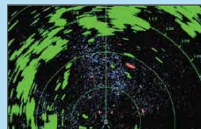
In the unique Rain Mode setting, rain cells are displayed as blue targets and lets you see through a storm cell to identify targets that would normally be hidden in the rain.
