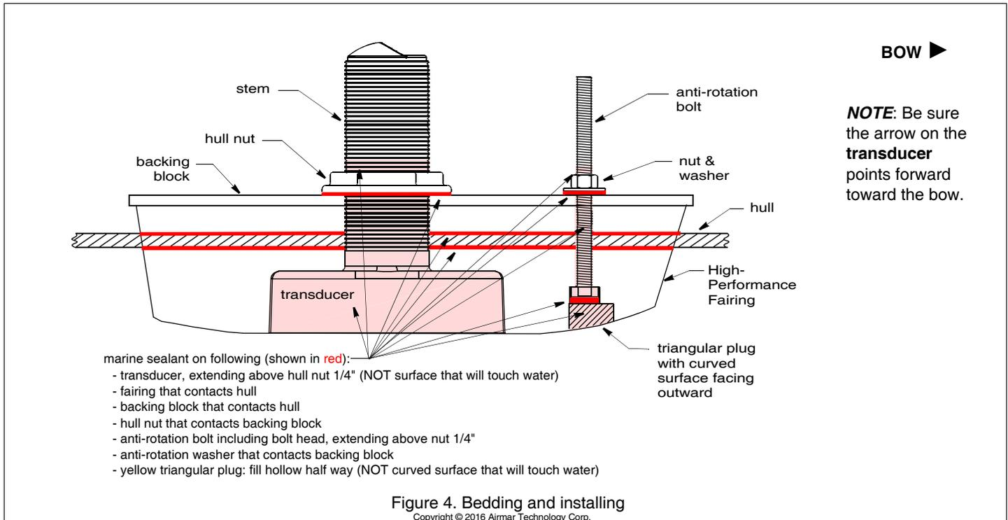
7. Check to be sure the transducer is flush with the fairing. If it is recessed more than 0.5mm (1/64") inside the fairing, you may shim the transducer or carefully file/sand the fairing.
