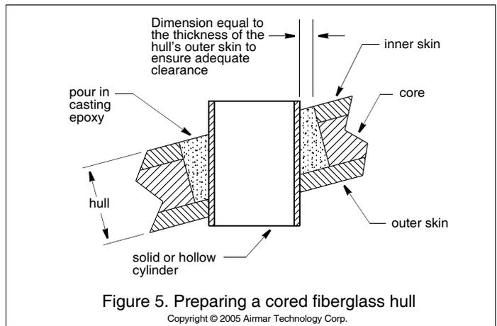
Using the appropriate size drill bit or hole saw, cut through the *inner* skin and most of the core from inside the hull keeping the drill perpendicular to the hull. The core material can be very soft. Apply only light pressure to the hole saw after cutting through the inner skin to avoid accidentally cutting the outer skin.
