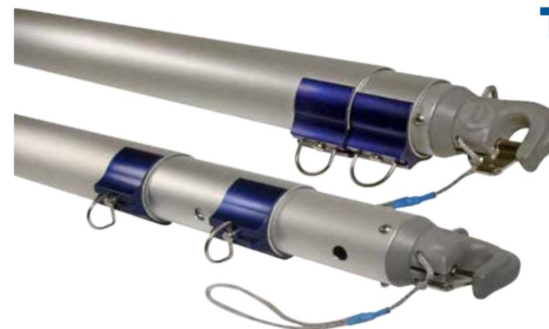
For use on boats 31 to 40 feet in length, the Tri-Reacher Whisker Pole was created to offer an affordable way to enjoy the performance benefits of an adjustable length whisker pole. This design uses large, easy to handle D-ring retention set pins for adjustment. Simply pull and twist the pin to hold it out, adjust the sections to the desired length and then reset the pin into the closest hole. Includes Ultra Series™ non-marring polymer pole ends.
