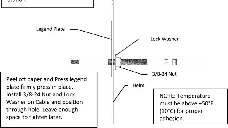
Peel off paper and Press legend plate firmly press in place. Install 3/8-24 Nut and Lock Washer on Cable and position through hole. Leave enough space to tighten later.
