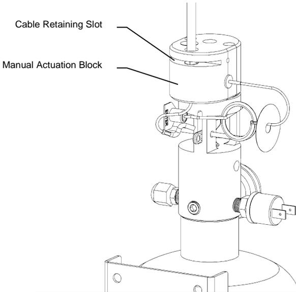
Insert extinguisher end of Cable through hole in Manual
