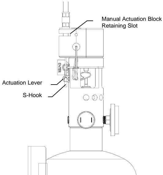
Align retaining slot of Cable with retaining slot of Manual Actuation Block.
