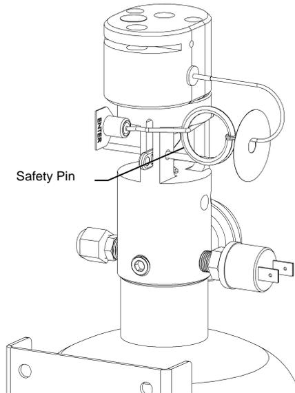
Extinguisher should be securely mounted and Cable should be routed.
