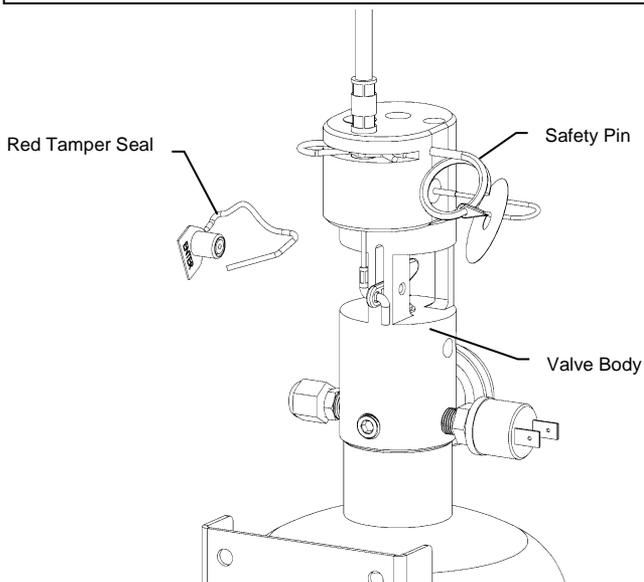
With T-Handle previously secured, remove Red Tamper Seal from Extinguisher to remove Safety Pin and store in provided hole. Cable system is now operational.
