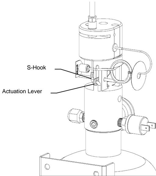
Insert S-Hook into hole of Actuation Lever.
