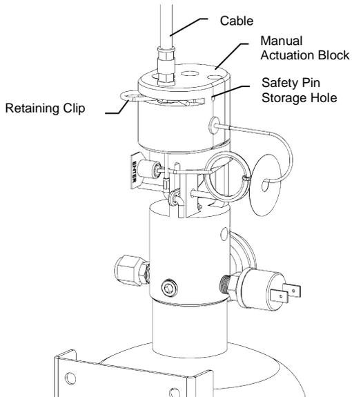
Secure Cable into Manual Actuation Block with Retaining Clip.
