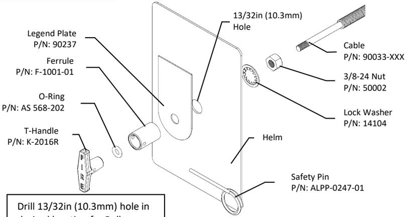
Drill 13/32in (10.3mm) hole in desired location for Pull Station.
