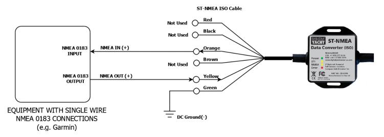
Below is a typical connection diagram for connecting the ST-NMEA Converter to a 2 wire NMEA0183 Devices, which are now what you will find in the majority of new systems and are fully NMEA0183 compliant.
