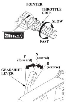
To shift gears, turn the throttle grip to the SLOW position; then move the gearshift lever to select the F (forward), N (neutral), or R (reverse) gears.
