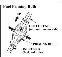
A priming bulb is built into the fuel hose that connects the fuel tank to the outboard motor.
