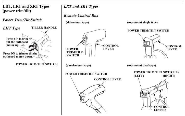
The power trim/tilt switch is located on the control lever. It is a rocker switch with UP and DN (down) positions for changing the angle of the outboard motor.
