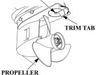
Adjust the trim tab with the engine stopped. Loosen the trim tab bolt above the trim tab, turn the trim tab, and then tighten the bolt securely.
