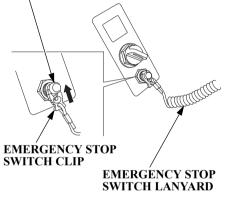
1. Put the emergency stop switch clip in the emergency stop switch, and attach the emergency stop switch lanyard securely to the operator or to the operator's PFD (Personal Flotation Device). The engine will not start or run unless the emergency stop switch clip is in the emergency stop switch.
