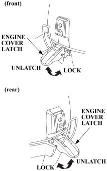
The engine cover latches fasten the engine cover to the outboard motor.
