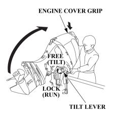
To tilt the outboard motor, move the tilt lever to the FREE (TILT) position, then raise the outboard motor to the desired position by pulling on the engine cover grip.
