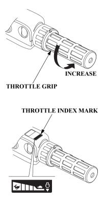
The throttle grip controls engine speed.
