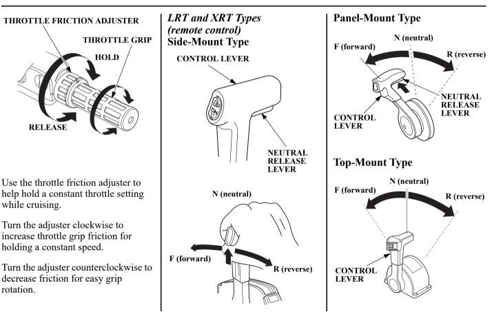
To shift gears, move the control lever to select the F (forward), N (neutral), or R (reverse) gear.
