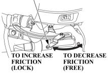
The steering friction adjuster adjusts steering resistance.
