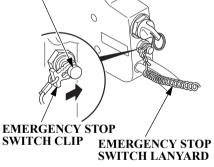
1. Put the emergency stop switch clip in the emergency stop switch, and securely to the operator or to the operator's PFD (Personal Flotation Device). The engine will not start or run unless the emergency stop switch clip is in the emergency stop switch.
