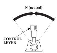
1. Move the throttle grip to the slowest speed and the gearshift lever or control lever to the N (neutral) position.
