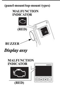
When the engine control system detects an engine control system malfunction, the malfunction indicator turns on and the buzzer sounds at one-second intervals.
