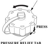
4. The fuel filler cap will lock again. Press down the pressure relief tab, and turn counterclockwise to remove the fuel filler cap.
