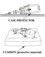
If it is necessary to store the outboard motor horizontally as shown, drain the vapor separator (p. 117), and drain the engine oil (p. 99), before removing the outboard motor from the boat.
