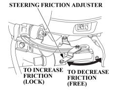
Tighten the steering friction adjuster to prevent the outboard motor from moving while trailering the boat.
