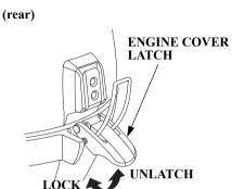
The engine cover latches fasten the engine cover to the outboard motor.
