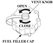
The fuel filler cap is provided with a vent knob to seal the portable fuel tank for carrying it to and from the boat. Open the vent by turning the vent knob counterclockwise all the way before starting the engine.
