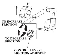
Adjust the control lever friction adjuster so the control lever will hold a constant throttle setting while cruising.
