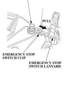
LRT and XRT Types (remote control) **Side-Mount Type** EMERGENCY STOP SWITCH PULL EMERGENCY STOP SWITCH CLIP EMERGENCY STOP SWITCH LANYARD **Panel-Mount/Top-Mount Types** EMERGENCY CONTROL PANEL STOP SWITCH EMERGENCY STOP SWITCH LANYARD PULL **EMERGENCY STOP SWITCH CLIP**
