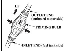
Hold the priming bulb up in the direction of the arrow; then squeeze the priming bulb several times until it feels firm, indicating that fuel has reached the engine.
