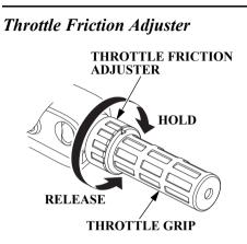
The throttle friction adjuster adjusts resistance to throttle grip rotation.
