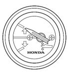
The trim meter indicates the relative trim angle of the outboard motor.
