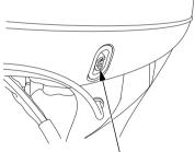
**POWER TILT SWITCH** (LHT, LRT and XRT Types)
