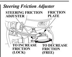
Use the steering friction adjuster to help hold a steady course while cruising.
