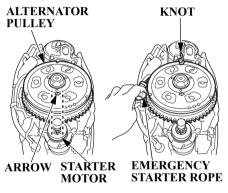
6. Set the alternator pulley so the arrow is lined up with the starter motor as shown. Hook the knot on the starter rope to the aft cutout as displayed above right. Wind the 160 cm starter rope (counterclockwise) 3 times around the alternator pulley.
