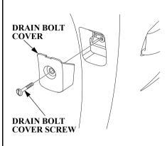
2. Loosen the drain bolt cover screw using a flat blade screwdriver and remove the drain bolt cover.
