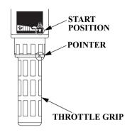
3. Align the engine start symbol "♂" on the tiller handle with the pointer "▶" on the throttle grip.
