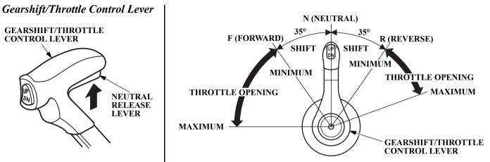
The gearshift/throttle control lever controls engine speed and selects F (forward), N (neutral), or R (reverse) gears.
