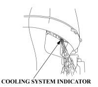
Water should flow from the cooling system indicator while the engine is running. This shows that water is circulating through the cooling system.
