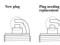
4. Inspect the spark plugs. Replace them if the electrodes are worn, or if the insulators are cracked or chipped.
