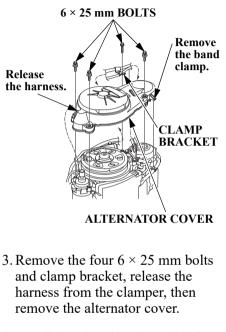
4. Install the clamp bracket with the  $6 \times 25$  mm bolt.
