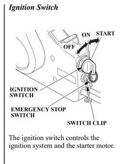
Turning the ignition switch key to the START position operates the starter motor. The key automatically returns to the ON position when released from the START position.
