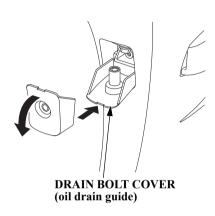
3. Place the drain bolt cover as shown to use it as an oil drain guide. Place a suitable container under the guide.
