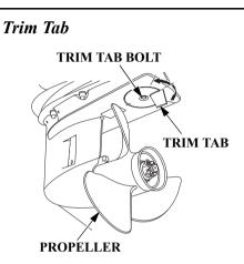
The trim tab compensates for "torque steer," which is a reaction of the outboard motor to propeller rotation.
