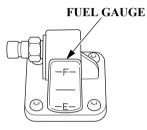
A fuel gauge is built into the fuel tank connector of the portable fuel tank.
