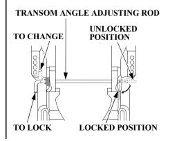
The transom angle adjusting rod limits the tilt angle of the outboard motor when fully lowered.
