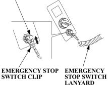
1. Put the emergency stop switch clip in the emergency stop switch, and attach the emergency stop switch lanyard securely to the operator or to the operator's PFD (Personal Flotation Device). The engine will not start or run unless the emergency stop switch clip is in the emergency stop switch.
