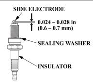
5. Measure the spark plug electrode gap with a wire-type feeler gauge. Correct the gap, if necessary, by carefully bending the side electrode.
