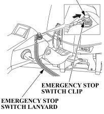
1. Put the emergency stop switch clip in the emergency stop switch, and attach the emergency stop switch lanyard securely to the operator or to the operator's PFD (Personal Flotation Device).
