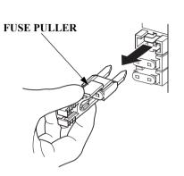
4. Use the fuse puller to remove the fuses. If a fuse is blown, install a replacement fuse of the same specified rating. The outboard motor is supplied with spare fuses in the fuse holder.
