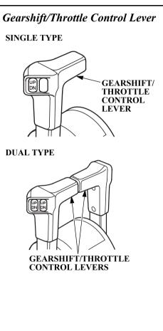
The gearshift/throttle control lever(s) controls engine speed and selects F (forward), N (neutral), or R (reverse) gears.
