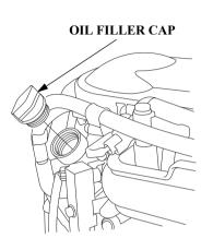
4. If the oil level is low, remove the oil filler cap, and add oil to reach the upper limit mark shown on the dipstick. Use the oil recommended on p. 101.
