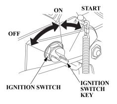
The ignition switch controls the ignition system and the starter motor. Turning the ignition switch key to the START position operates the starter motor. The key automatically returns to the ON position when released from the START position.
