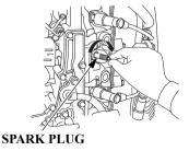
6. Install the spark plugs carefully, by hand, to avoid cross-threading.
