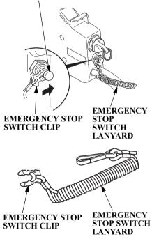
The emergency stop switch clip must be inserted in the emergency stop switch in order for the engine to start and run. The emergency stop switch lanyard must be attached to the operator's PFD (Personal Flotation Device) or to the operator securely.
