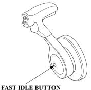
Use the fast idle button to accelerate engine warm-up after starting the engine. Do not use the fast idle button when starting the engine.
