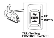
TRL (Trolling) Control Switch Panel [optional equipment (except LHA and LHTC types)]
