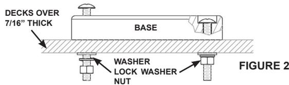
**Decks Less Than 1/4" Thick:** To prevent deflection and add stability to decks thinner than 1/4", we recommend using a Cannon Deck Plate (part no. 2200693). To mount the Deck Plate, use it as a template to mark hole locations. Fasten it to your boat with four 1/4"-20 flat head machine screws with wellnuts, if you cannot access the underside of the deck, or with washers and nuts if you do have access under the deck (see Figure 3).
