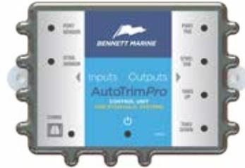
The ATP Control Unit is the sensor and processor for the ATP system which activates the electric actuators that adjust the trim tabs. The unit contains an accelerometer, gyroscope, and an electronic compass that sense the position and movements of the boat and therefore should not be mounted within 24" of any magnetic items such as electric motors or speakers. However, the ATP Control Unit can be conveniently mounted anywhere in the boat, and in any orientation.
