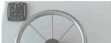
the operating position. Ideally, the ATP Helm Display should be installed in a horizontal position. This makes the use of the control more intuitive. It is important for the vessel operator to be able to clearly see the LED indicators on the ATP Helm Display to know what the ATP is doing.
