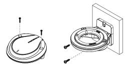
1. The compass can be mounted directly to a flat surface, or using a wall bracket.
